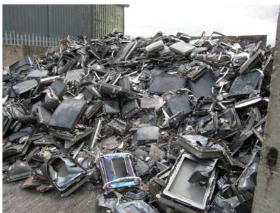
Figure 3 - open storage of broken CRTs is unacceptable
